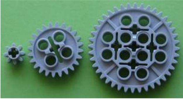
These gears have 8, 24 and 42 teeth (*one of these numbers is wrong – find the gears and count the teeth to see which count is incorrect*).
