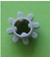
The small driving gear is now added to the Robot. Note that it may be necessary to wiggle the gears to help fit this gear in to the place shown in the image below.
